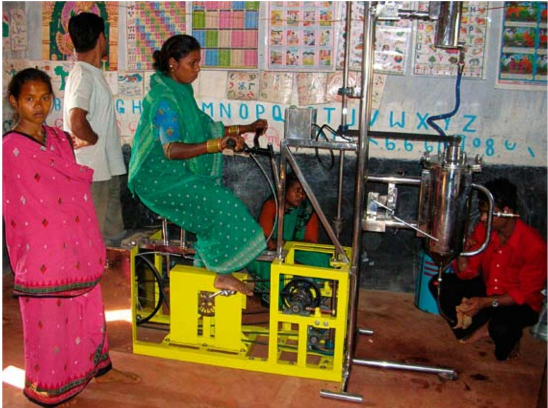
Photo: Pedal-driven Biodiesel Reactor; CTxGreEn
