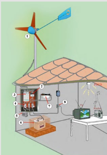
Fig. 3: Schematic view of a wind power system for off-grid applications
