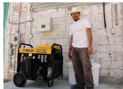
One of the farmers using a gasoline motor modified to run on biogas
